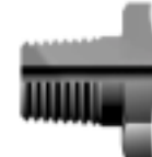
M -ANSI/ASME B1.20.1 External pipe threads
